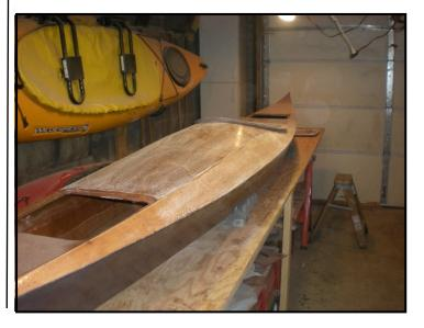
The answer of course is wood - specifically, marine plywood sheathed in fiberglass and epoxy.
